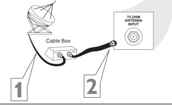
Your Cable Box may have separate Audio and Video Out jacks instead. If so, use audio and video cables to connect the AUDIO /VIDEO OUT jacks of the Cable Box to the AUDIO/VIDEO IN2 jacks on the rear of the TV. Press the TV/AV on the remote control to set the TV to the AV2 channel. Change channel at the Cable Box.
